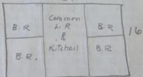
These buildings consist of shiplap walls and floor and common lumber roof covered with rubberoid. Outside walls and floor also covered with rubberoid. Inside walls not sheeted but covered with light-coloured building paper glued on.
